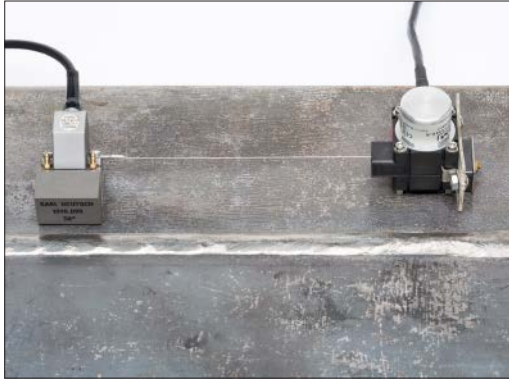
Wire encoder with magnetic foot, scan length 500 mm, 40 pulses/mm, order no.:1885.002
