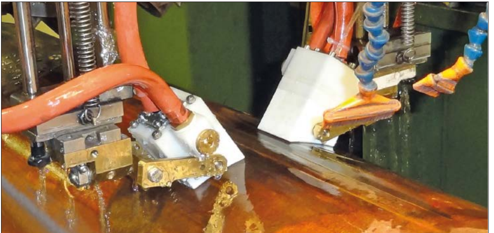
Water nozzle for probe 1598.666 and 1598.649 with customized radius, e.g. for mechanized testing of longitudinal tube welds
